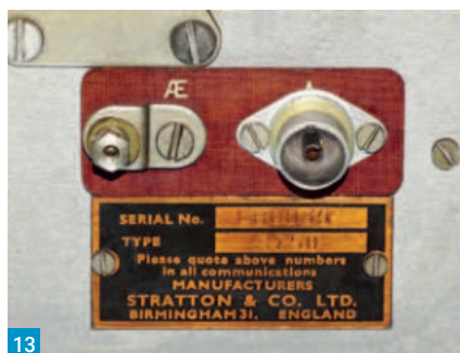
Fig. 13: For use as a tuneable IF, the original antenna input terminal should be replaced by a coax socket.
