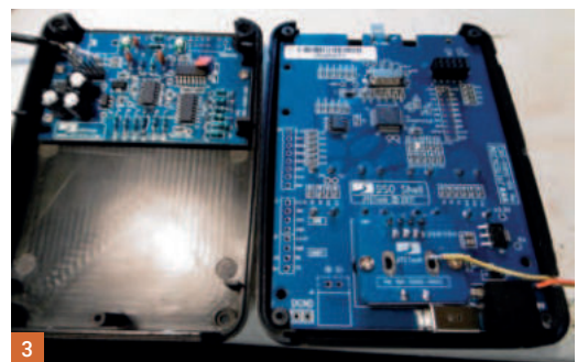
Fig. 1: The kit. The surface mount components arrive already mounted and soldered.
