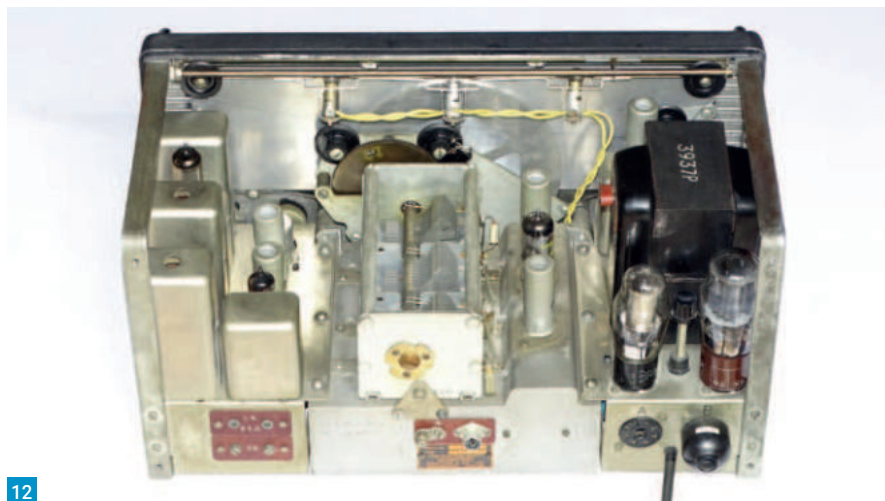
Fig. 12: The heart of the S750 is a diecast coil box, which is rigidly secured to the front panel and flanked by a pair of nickel-plated brass subchassis carrying the IF and AF stages, the power supply and the BFO.
